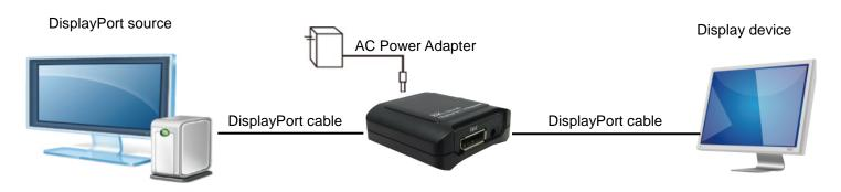
The 8K DisplayPort 1.4 Repeater is installed between the DisplayPort source and a connected DisplayPort monitor.
