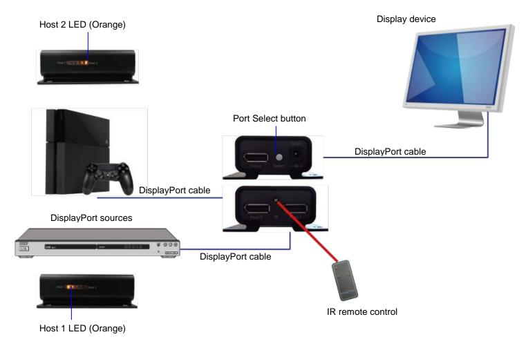
Fig. 1 The 2-Port DisplayPort switch is installed between the DisplayPort sources and a connected DisplayPort monitor.
