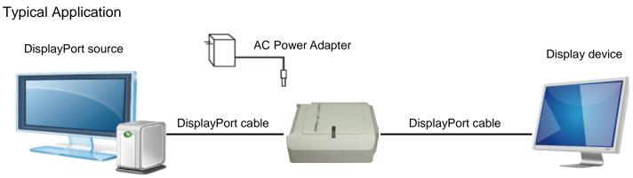
The DisplayPort Repeater is installed between the DisplayPort source and a connected DisplayPort monitor.
