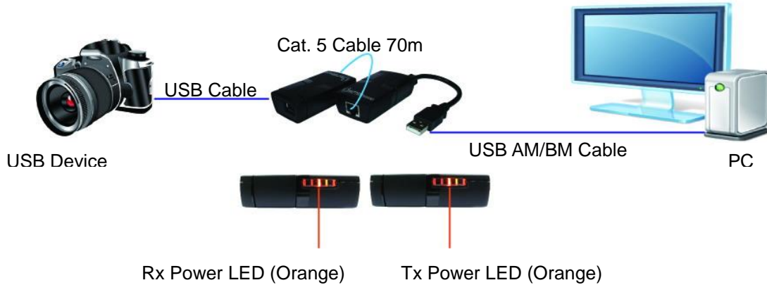
Fig 1. The USB 2.0 Extender is installed over Cat.5 cable between the PC and a connected USB device.
