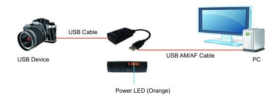
Fig 1. The USB Isolator unit is installed in-line between the PC and a connected USB device.
