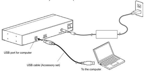
(7) In according to the previous instruction of connection with host computer, and connects host computer with the unit.
